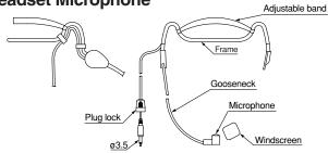
WH-4000A is headset microphone of a cardioid pick-up pattern, featuring a lightweight design.
