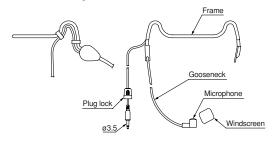
WH-4000H is headset microphone of a cardioid pick-up pattern, featuring a lightweight design.
